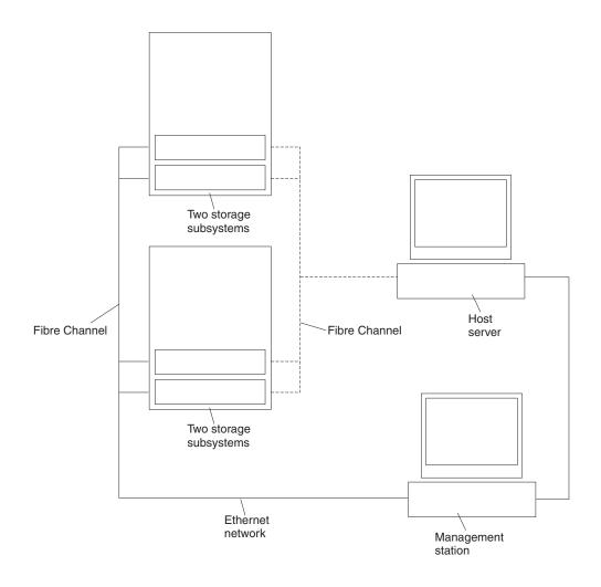
Figure 53. Direct (out-of-band) managed storage subsystems
